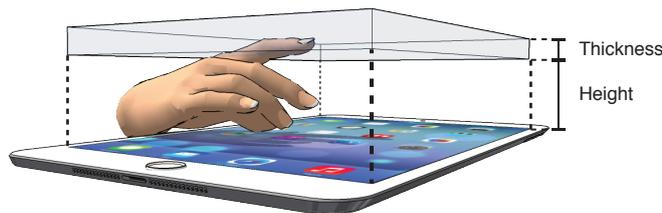
**Figure 4.1:** A schematic of a near-surface input layer
