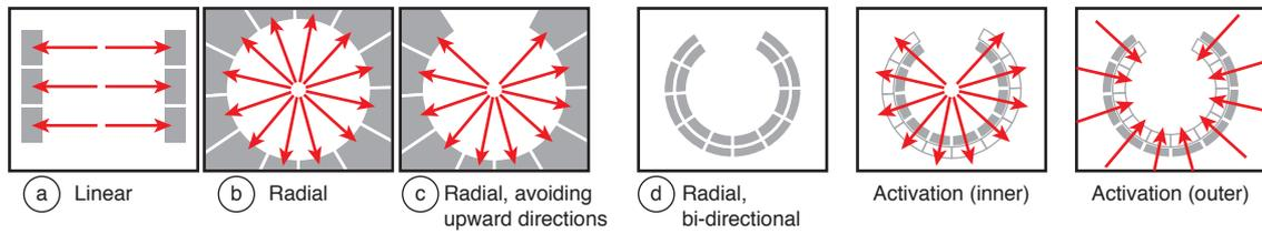
**Figure 2.7:** Target layouts for swabbing. Each of the filled grey shapes is a target. To activate each target, users perform swabbing gestures roughly in the direction pointed by the red arrow intersecting each target.
