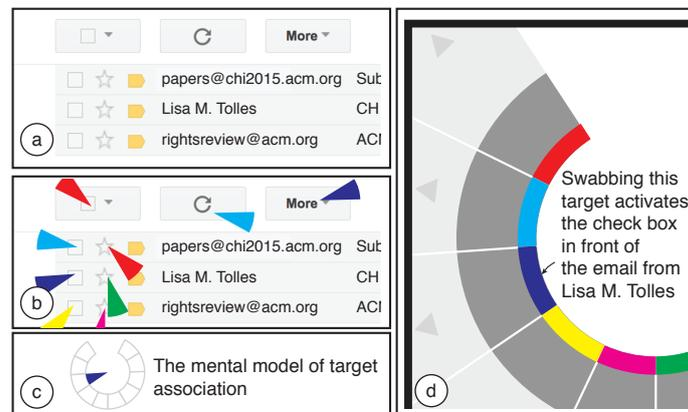
**Figure 2.9:** How swabbing visualize the association between swabbing targets and the original UI widgets. (a) A screen of an email application with several UI widgets of the same type. (b) Target pointers pointing to different directions. Adjacent directions are coded in different colors. (c) The mapping between the pointers and the swabbing target. (d) Swabbing user interface showing the corresponding swabbing targets.
