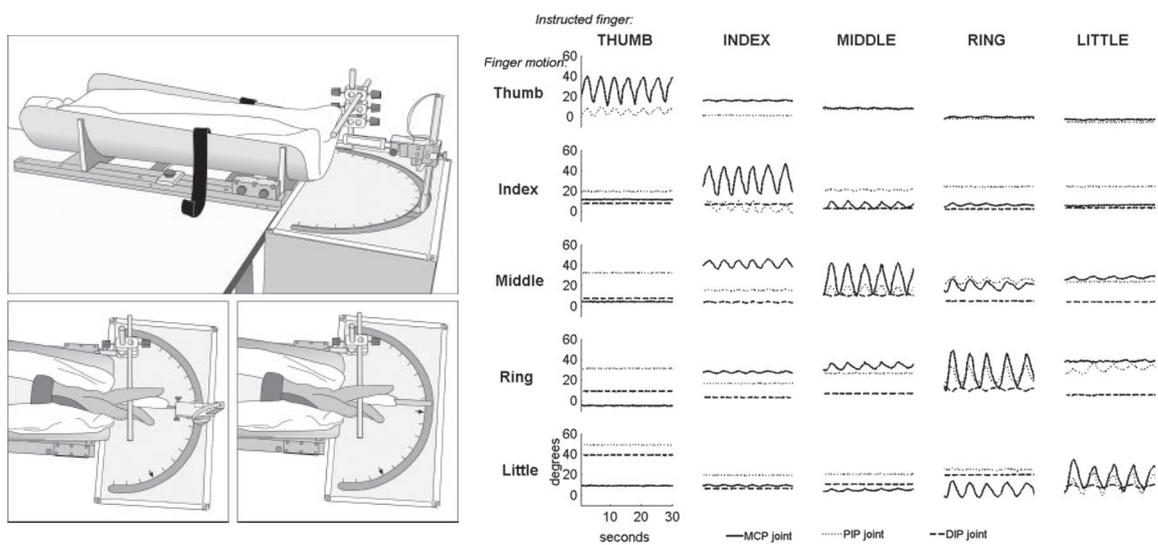
**Figure 1.4:** An experiment on mechanical coupling among fingers. Left: a schematic of the device used to measure the coupling. Right: A trace of finger movement. The presence of movement amplitude apart from the cells on the main diagonal indicates coupling. (Image adopted from Lang and Schieber [2004])
