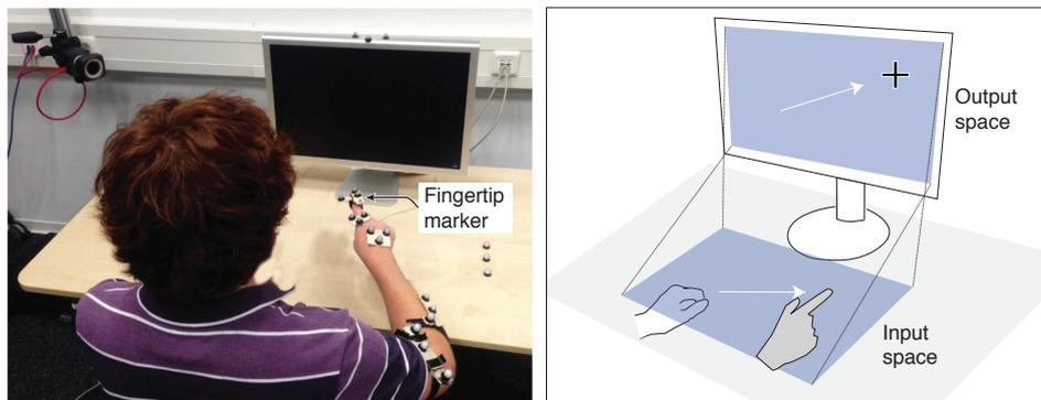
Figure 4.4: The hardware setup for our user studies (left), and the cursor mapping (right)<sup>1</sup>.
