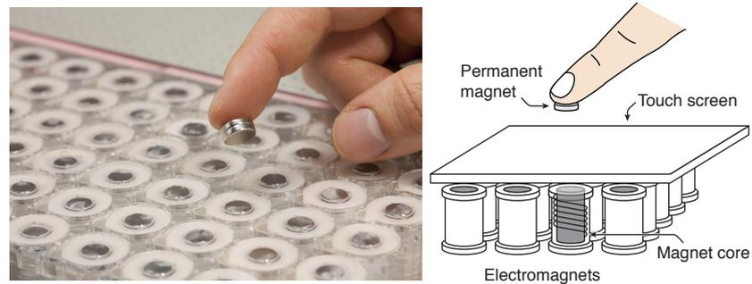
**Figure 5.2:** The FingerFlux prototype. An array of electromagnets, placed below a touch screen. Powering these electromagnets creates a magnetic force field that attracts or repels the permanent magnet at the fingertip. (Left image courtesy of [Weiss et al., 2011])
