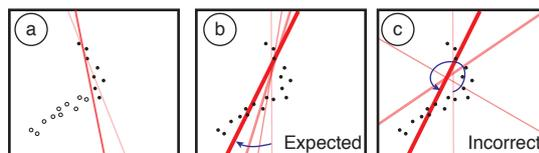
**Figure 2.10:** Swabbing crossing the Y-axis may result in unexpected visual feedback. (a) The touch trace of a swabbing from top to bottom. Filled dots are the touches that already occur. Blank dots are the touches to occur. The red lines show the regression. Recent regressions are thicker and more opaque. (b) The expected rotation. (c) The rotation in the opposite direction.
