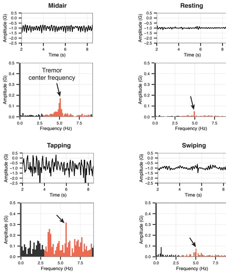
**Figure 2.4:** Examples of accelerometer data (top panels) and their Fourier transformation (bottom panels). The amplitudes in the tremor frequency range was increased by tapping, but swiping yields relatively low amplitudes. The frequency region we used in the analysis is highlighted. All data shown here were captured from the same participant (moderate tremor).
