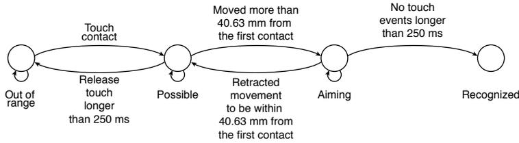
**Figure 2.6:** The state model of the swabbing gesture recognizer.
