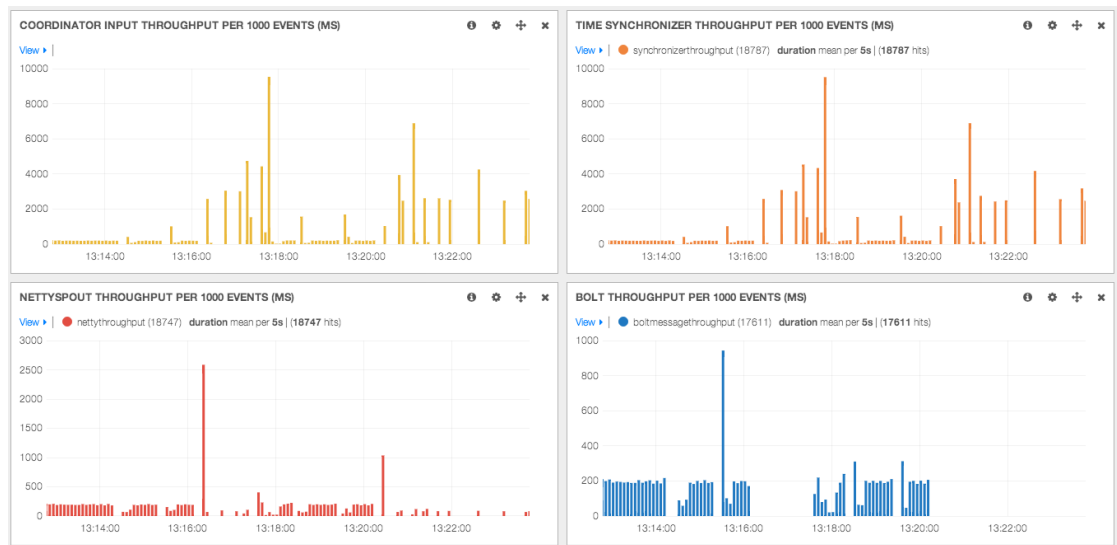
Figure 4.21: Speed layer monitoring: The graphs show histograms of the average time it takes to process messages at different components of the architecture. From top left to bottom right: (i) input reader (ii) time synchronizer (iii) NettySpout and (iv) Bolt.
