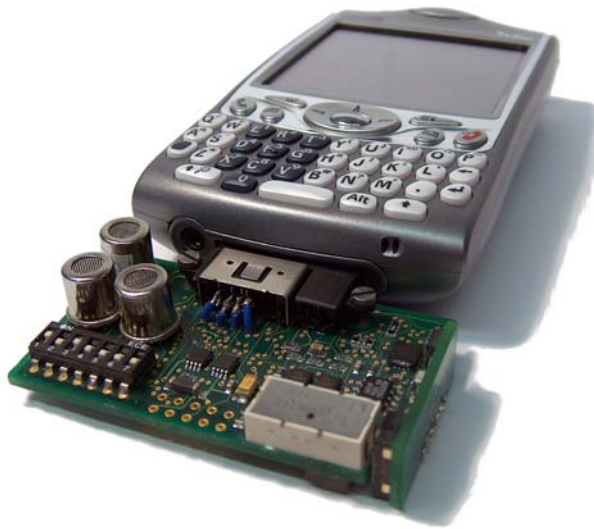
Figure 1: The Treo 650 smartphone with attached sensorboard
