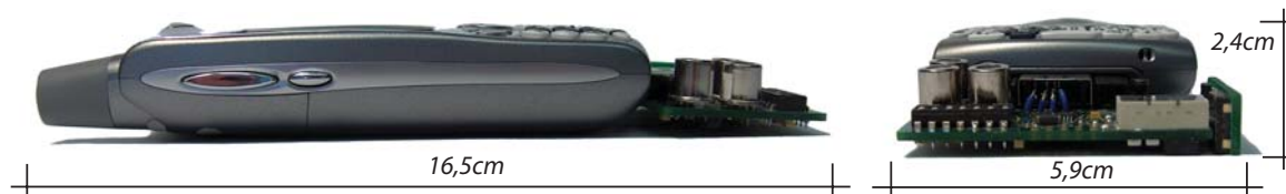
Figure 6: The sensorboard attached to the smartphone via the multi-connector
