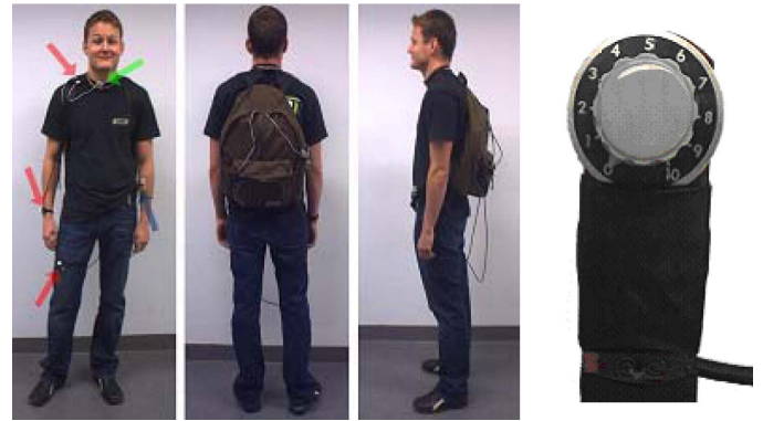
Fig. 1. a) Subject wearing data acquisition setup with accelerometers (red arrows, left side of figure), microphone (green arrow, top right side), and potentiometer (blue arrow, bottom right side). b) Potentiometer only on the left.
