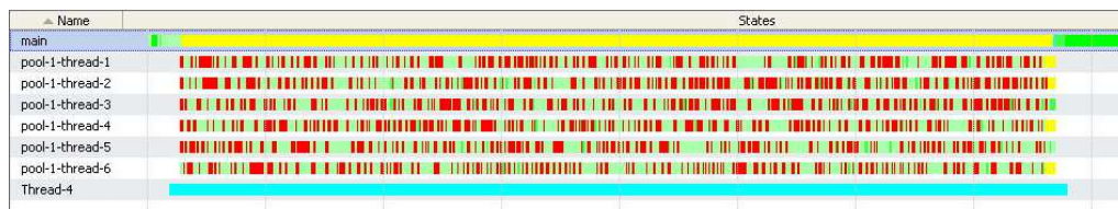
Figure A.10: Thread view of the threaded DB-based expander influenced by a 10Mbit LAN and permanent packet collisions.
