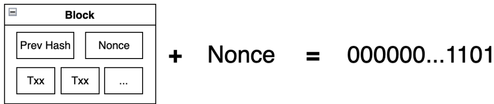
Figure 3.2: Latest block plus a Nonce create SHA-256 Output with 6 leading Zeros
