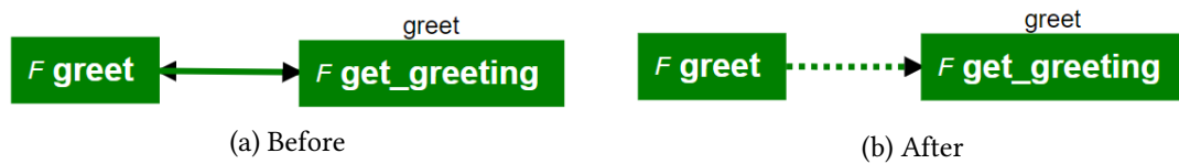
Figure 11: Function greet with a nested function get_greeting , which gets called by greet . To prevent confusion, only the calling relation is shown with a link, with the parent relation being signified by the parent's name on top of the child node.
