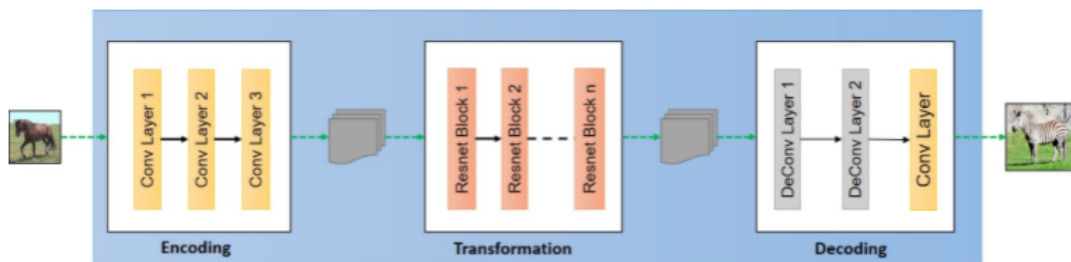
Figure A.4: Schematic representation of the CycleGAN ResNet-based generator. In contrast to the U-Net configuration, the ResNet has a "flatter" architecture, as the skip connections are retained in the transformation part. The first step, encoding, consists of extracting features from an image, which is done using a convolutional network. The goal of the transformation is to retain the features of the original input, such as the size and shape of the object, so ResNet is well suited for this type of transformation. Decoding is similar to the U-net and aims to reproduce the image in the same size. Source: CycleGAN blog Hardik Bansal (2017)
