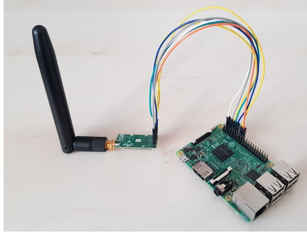
Figure 4.3: Raspberry Pi 3B with the E32-868T20D attached.
