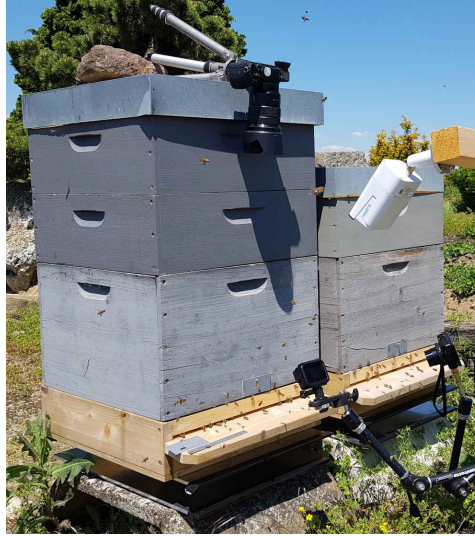
Figure 17: Camera setup. We used the video material from the three black cameras for evaluation. The white camera surveils the hive permanently and its footage was not included in the evaluation. Source: Daniel Boschung
