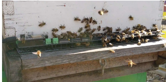
Figure 9: Bee counting with optical sensors [36]
