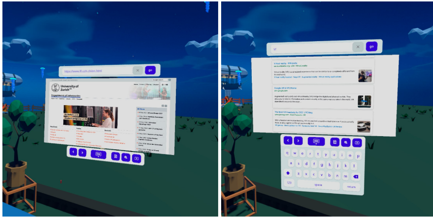
Figure 4.19: The VR web browser being used in a virtual work oasis. The custom user interface surrounds the browser window. The onscreen keyboard can be seen in the image on the right.
