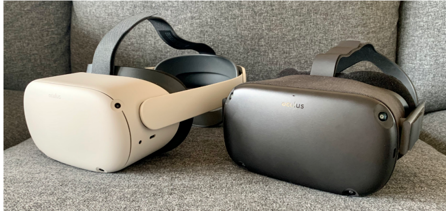
Figure 3.1: The Oculus Quest line of headsets, with the Quest 2 on the left and the original Quest on the right.
