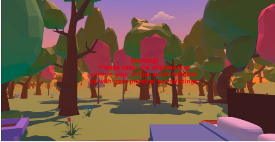
Figure 4.4: The warning message shown to the user if Holoft detects a possible issue with the alignment. This message is overlaid onto everything and moves with the headset.
