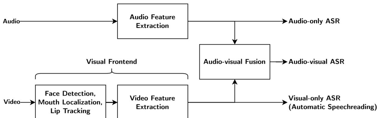
Figure 2.3: The main building blocks of an audiovisual automatic speech recognizer as described in [Potamianos et al., 2012].
