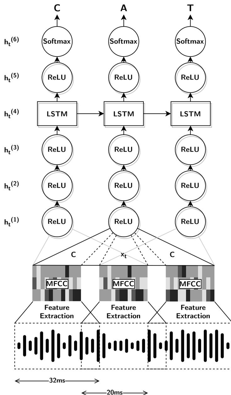
Figure 2.2: Architecture of Mozilla Voice STT (Adapted from [Hannun et al., 2014]).
