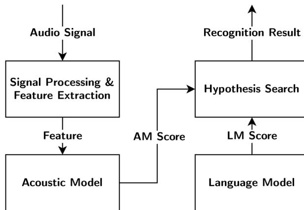
Figure 2.1: Architecture of *ASR* Systems [Yu and Deng, 2015].
