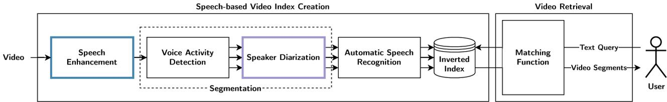
Figure 5.1: Overview of our speech based video retrieval prototype.
