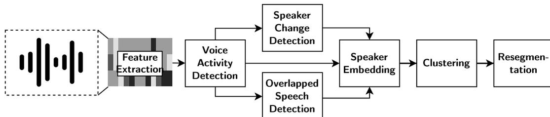
Figure 2.4: Speaker diarization pipeline as described in [Bredin et al., 2019].
