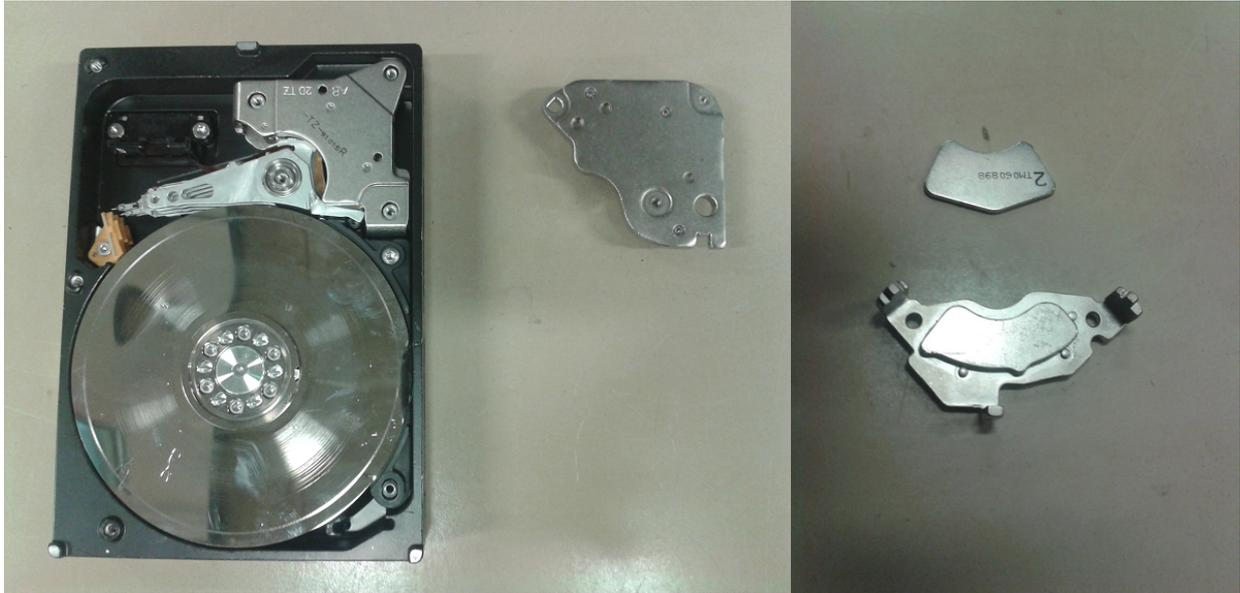
**Figure 2.3: Hard disk with neodymium-iron-boron magnets<sup>1</sup>**
