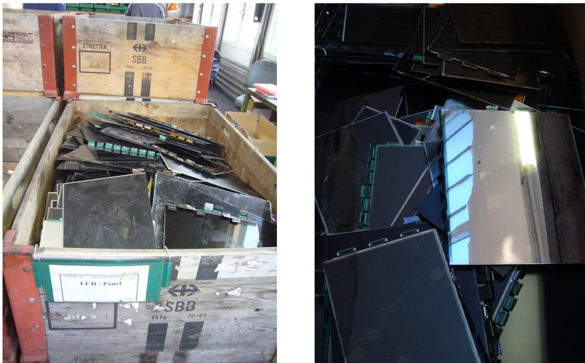
Figure 2.2: LCD panels resulting from manual dismantling<sup>1</sup>
