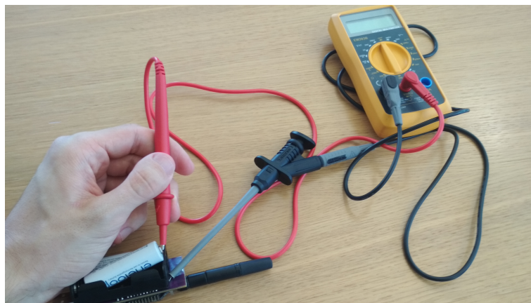
Figure 5.1: Energy consumption measurement setup [31]
