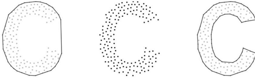
Figure 34: “C-shape” distribution approximated with Convex Hull (left) and Concave Hull (right) [8].
