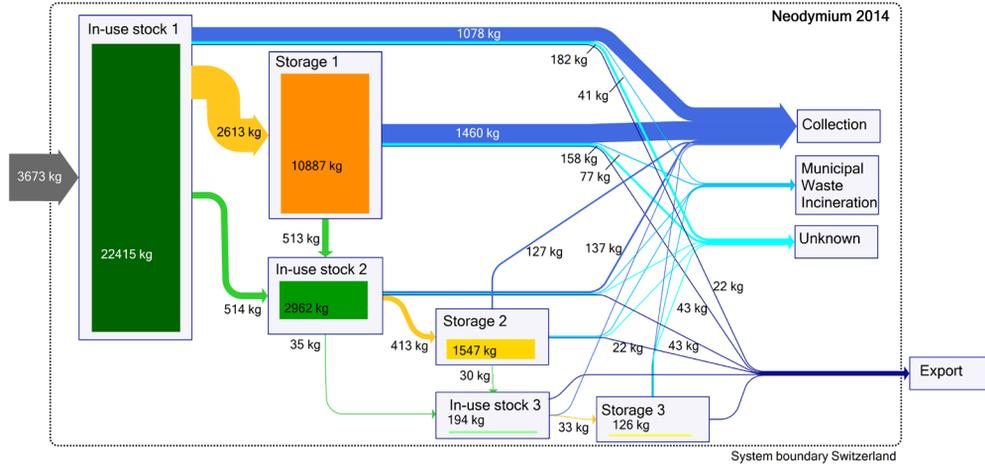
Figure 3: Nd flows in kg in 2014. Flows <20kg are not labeled.
