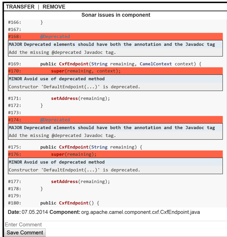
Figure 3.14: Data set showing code with marked Sonar issues. Sonar issues are marked red in the code. The description of the issue is displayed below the marker. The issues and the component name can be clicked in order to display the value context menu.
