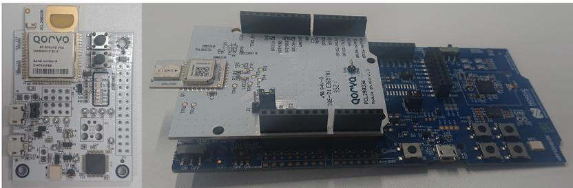
Figure 4.1: Left: DWM3001CDK. Right: nRF52840 and DWM3000EVB.
