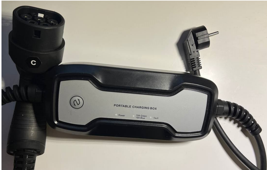
Figure 3.1: Morec portable home 3.6kW EV charger
