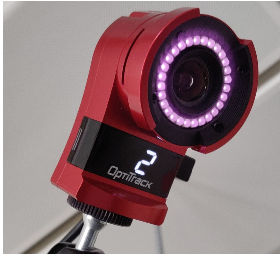
Figure 3.3: The Flex 13 camera used by the OptiTrack system, showing the illuminated LED ring around the lens which emits the infrared light used to track the markers.
