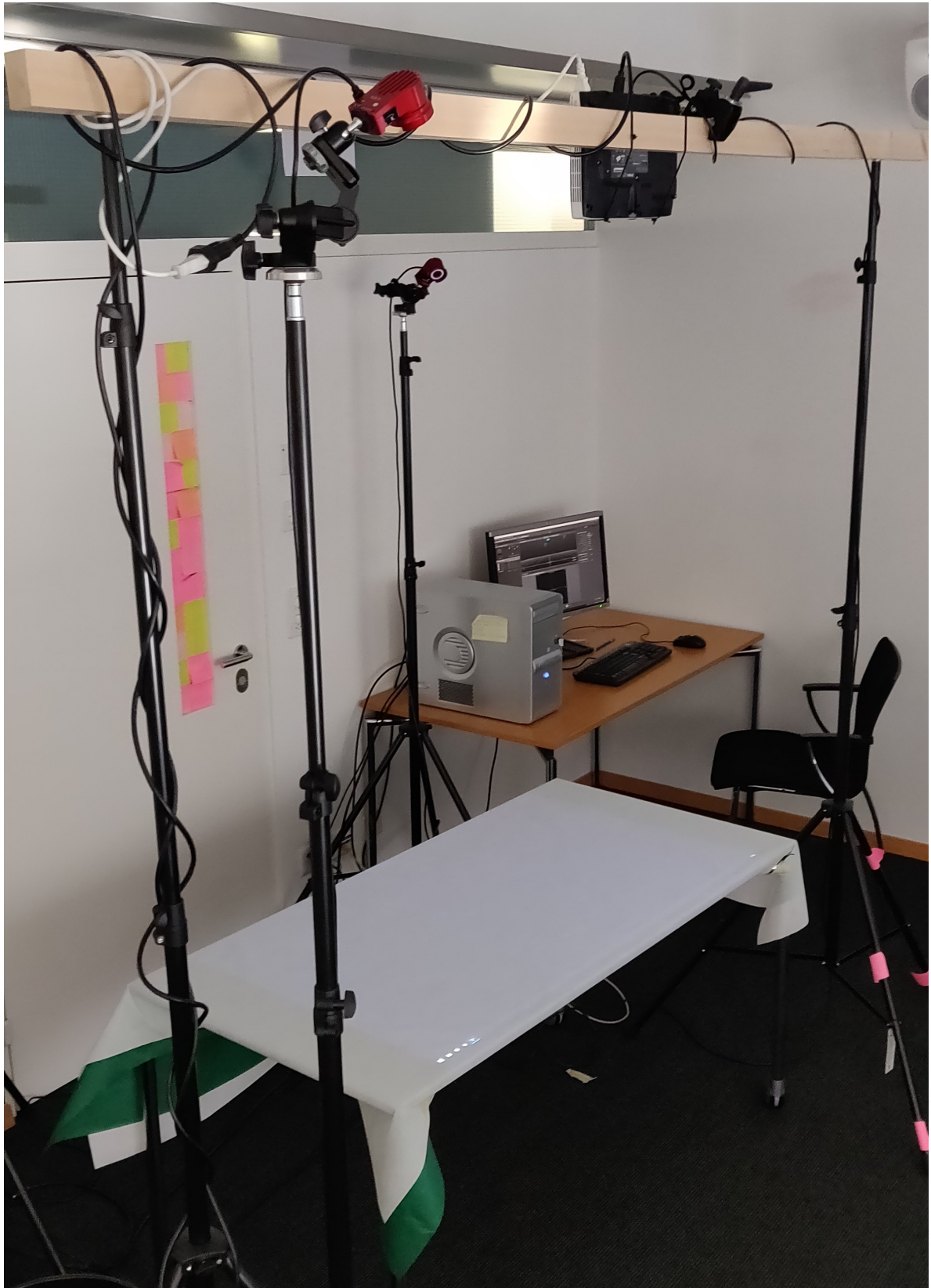
Figure 3.2: The OptiTrack system setup in the ZAPC Lab at the University of Zurich, showing the positions of the cameras used for tracking the retro-reflective markers.
