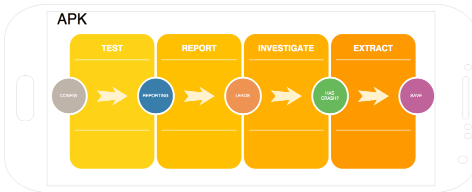
Figure 3.2: Approach performed by BECLOMA for testing a single Android app
